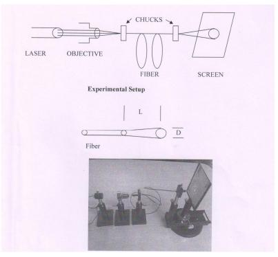
Fig. 1: Experimental setup for NA measurements
