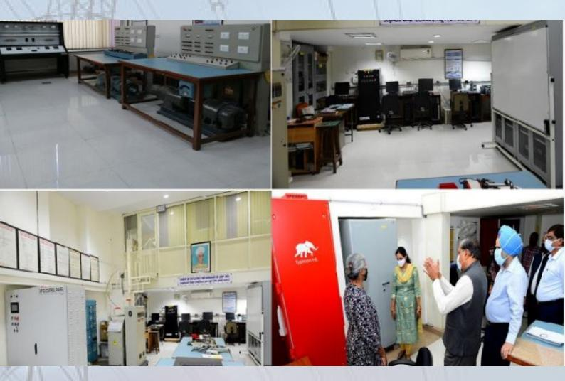
In addition to various conventional ac and dc machines, one set of universal machine is also available in the laboratory. A part of the Electrical Machines Laboratory is specifically developed for Contactor Control of Electric drives wherein various trainer boards have been developed for performing different exercises in this area.
