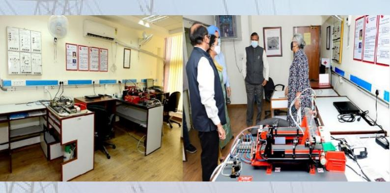
The PLC laboratory is equipped with PLC based control system and Advanced PLC Trainer; other interfacing devices to train students how to program and upload ladder logic code. The lab is based primarily on the Allen Bradley family of Programmable Logic Controllers, which are widely used in factories and other settings
